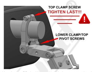
7 - At this point your RD should be positioned where you want it and the screws should be snug. Slightly loosen the top clamp screw so both the lower clamp/top pivot screws can be fully tightened. Grab the long arm of the allen wrench to assure that these screws are securely tightened, you will not strip out the tapped holes in the aircraft grade aluminum.
